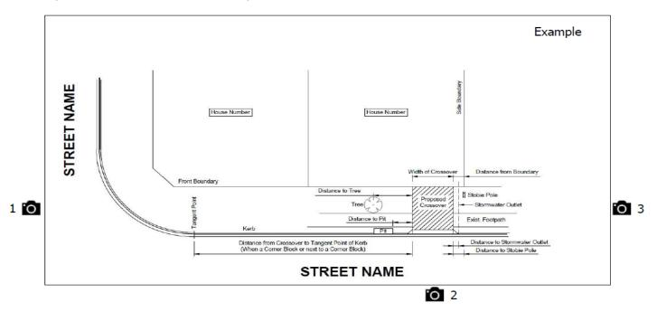
Photos of existing infrastructure should be taken from the 3 points as indicated above. The photos should capture all of the infrastructure indicated within the drawing.
